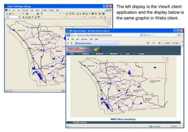
The ClearSCADA Web server defaults to the IP address of the ClearSCADA server and supports XML and/or html with optional secure sockets (SSL) for added security if necessary.
