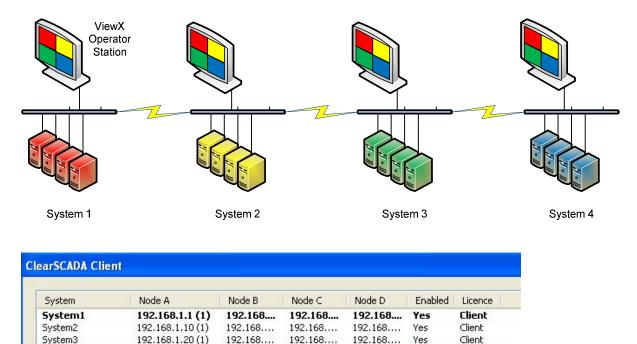
The ability for ClearSCADA server to be sized up to 250k points, multiple servers for redundancy and that operator workstation can connect to multiple systems simultaneously provides virtually unlimited scalability for ClearSCADA.
