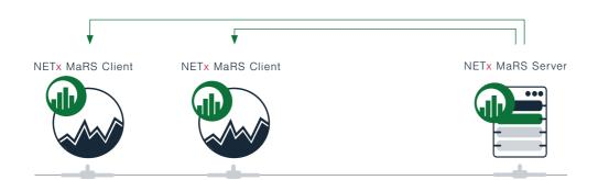
A NETx MaRS Client is an application program that performs different energy management tasks (e.g. visualization of the consumption values, calculation of the costs for each cost center, comparison and analysis of consumption values and costs, ...). A NETx MaRS Client acts as an application that is dedicated to the end user. In order to perform energy
